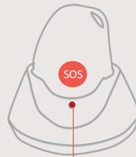
6. RED LED ON, THE GPS DEVICE IS CHARGING CORRECTLY
